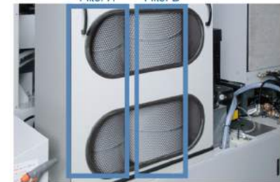
Filter automatic switching Switching the filters to be used automatically according to the filter pressure.(4-piece filter specification is necessary)
